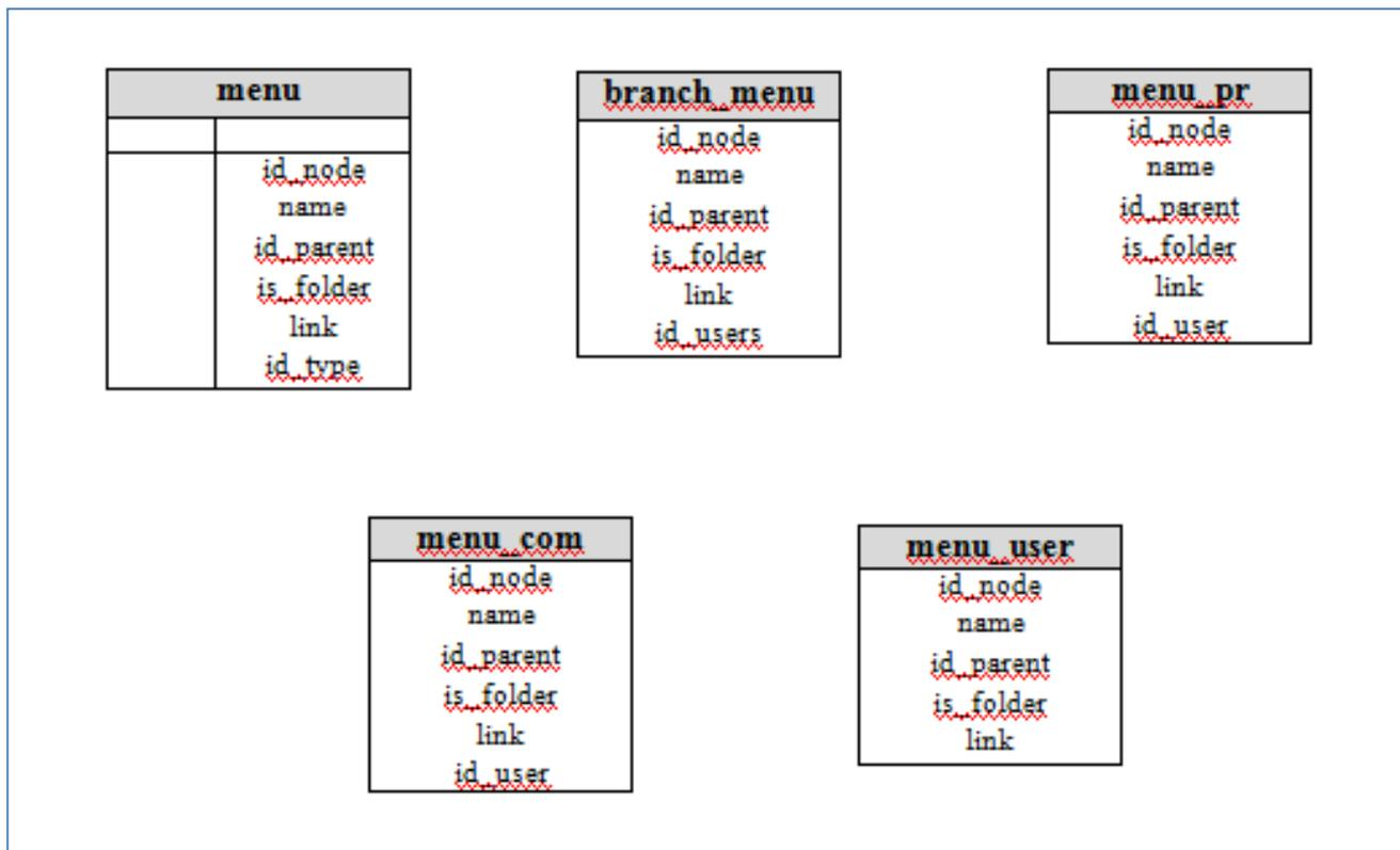
Figure 2 - Database objects that are used to build the menu
